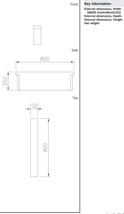
Modular Cooking Range Line thermaline 80 - 100 mm Closed Work top, 1 Side
